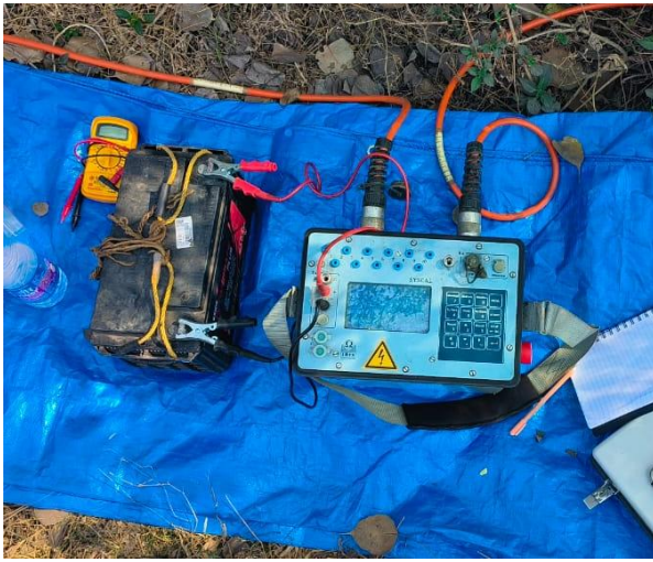
Detection of old and abandoned mine workings status over Sijua, Colliery, Jharia, Tata using Electrical Resistivity Tomography
